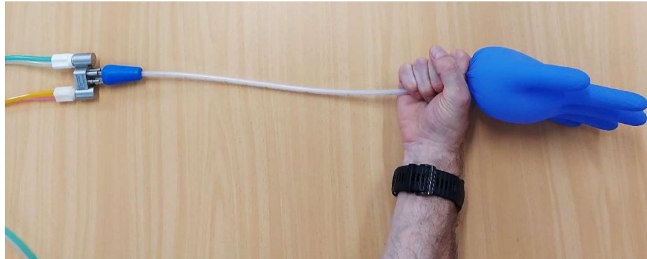
Figure 6: Pressure test. Ventilation is running. Glove inflates.
