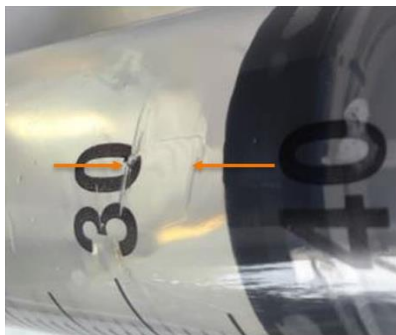
Figure 1: Example of syringe barrel damage on BD Plastipak™ 50mL Syringe with Luer-Lok™ Tip
